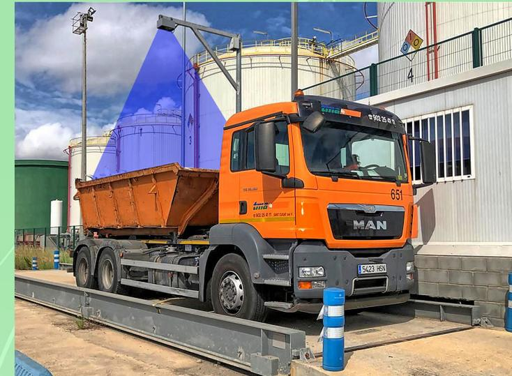
Measurement of the volume of ship waste – © goClever
